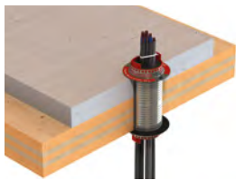
The Hilti CFS-SL GA fire safety sleeve is convenient for situations where cables often have to be relaid. It is ideal for office buildings or hotels in which electrical installations are regularly updated.
